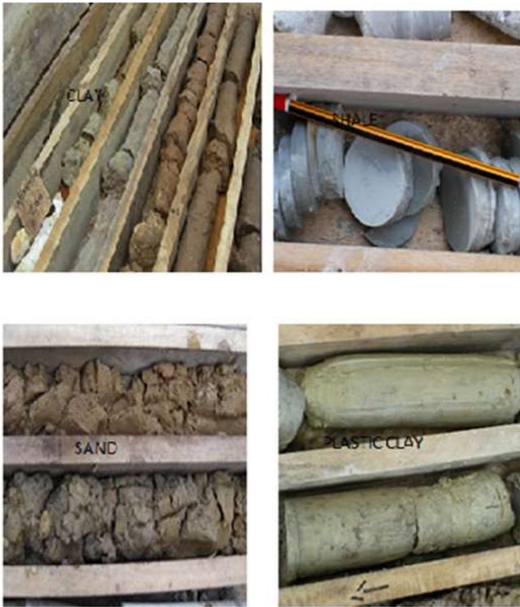
Fig 6-9: X-lithological samples of marl, shale, sand and clayey-shale sediments from the study area
