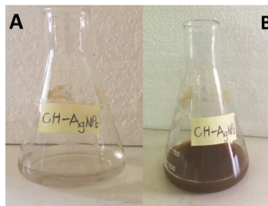
Figure 1: Synthesis of the Coconut husk extract mediated silver nanoparticles (a) immediately after the addition of the coconut husk extract to the silver nitrate; (b) Formation of deep brown colouration after 30 min.
