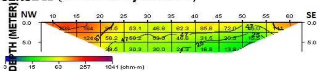
Figure 5: Inverted 2D sections beneath NW-SE traverses north of the dumpsite
