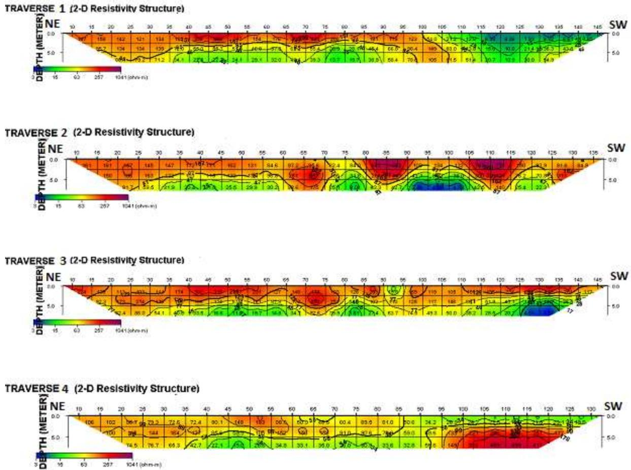
Figure 2: Inverted 2D sections beneath NE-SW traverses east of the dumpsite
