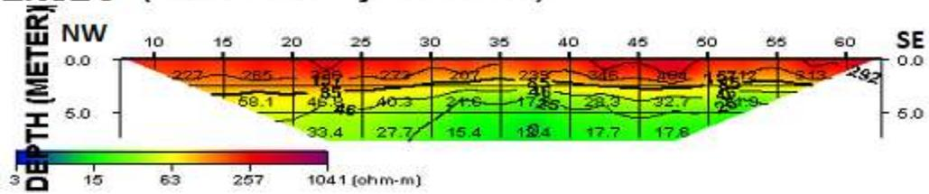
Figure 4: Inverted 2D sections beneath NW-SE traverses south of the dumpsite
